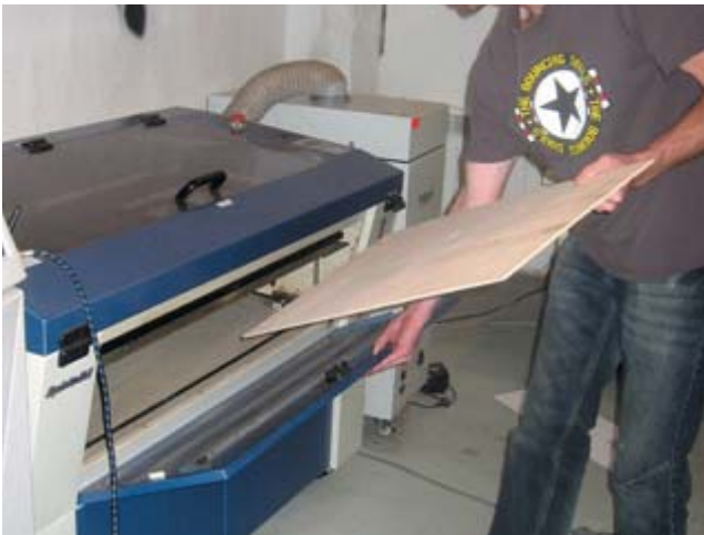
Larger non-flexible pieces should be placed in the bed through the removable front door.
