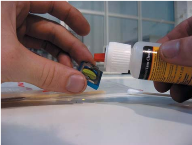
11. Use the lens cleaning solution and place a drop on the lens, or wet the swab.
