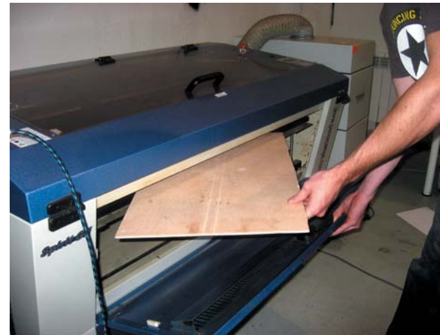
Placing plywood in the bed.
