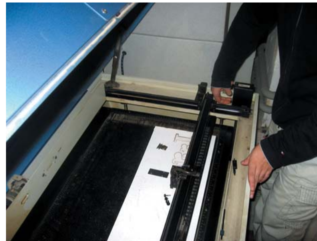
14. Put the mirrors and lens back in their original positions.
