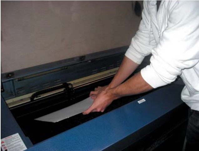
Smaller more flexible pieces can be placed in the laser bed from the top.
